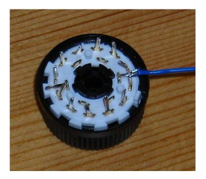
By careful bending of the legs and with a wire soldered to the selector connection it can be fitted to normal stripboard. It is large enough to be operated by a thickly gloved hand and the position felt as it clicks, and small enough to be stuck on the front of a Kobo.
