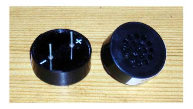
These are quite expensive but cheaper versions are available such as the Ekulit AL-23P. They are both 23mm in diameter and inside the housing is a 19mm diameter speaker.
