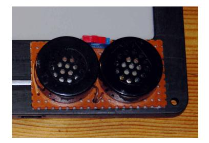
On this Kobo the speakers are mounted on a piece of stripboard fixed with double sided foam tape. There is also a small pcb slide switch visible at the top to switch the audio on and off.
